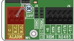
The operation modes that can be selected: Production, Alarm, Alarm Configurable, Crepuscolar, Alarm Configurable Latch, Alarm Configurable ext, GoGo relè (Auto), GoGo relè (Remote). Refer to the product manual for further details on the operation modes of the Alarm terminal.
