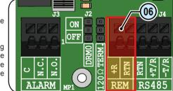
Where required, it is possible to activate the DRM0 function by configuring the Jumper for the activation of the DRM0 function (3) in the "ON" position
