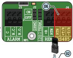
The last inverter of the daisy chain must be "terminated". Apply the 120 Ohm termination resistance by configuring the RS485 Line Termination Jumper @ to the "ON" position.
