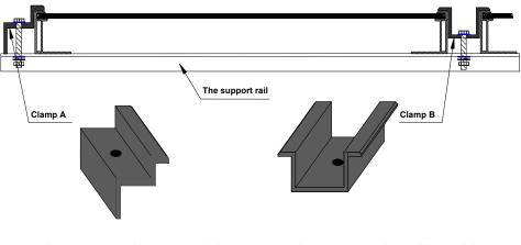
Clamp A: Fasten the Fringe modules Clamp B: Fasten the Middle modules
