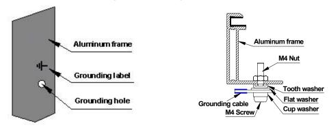
FIG 4 Grounding hole and ground label
