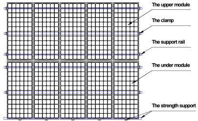
FIG 2 Schematic diagram of reinforcement mounting of module
